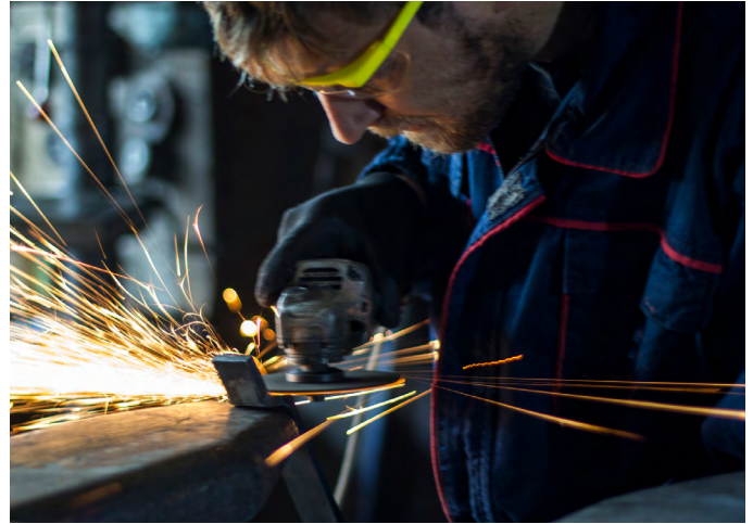
Grinding is an often overlooked hot work activity
