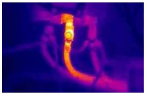
The above photo shows the same lead in operation at 320° F.
