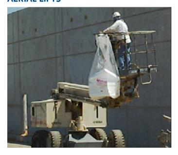
An aerial lift is any vehicle-mounted device used to elevate personnel, including:
