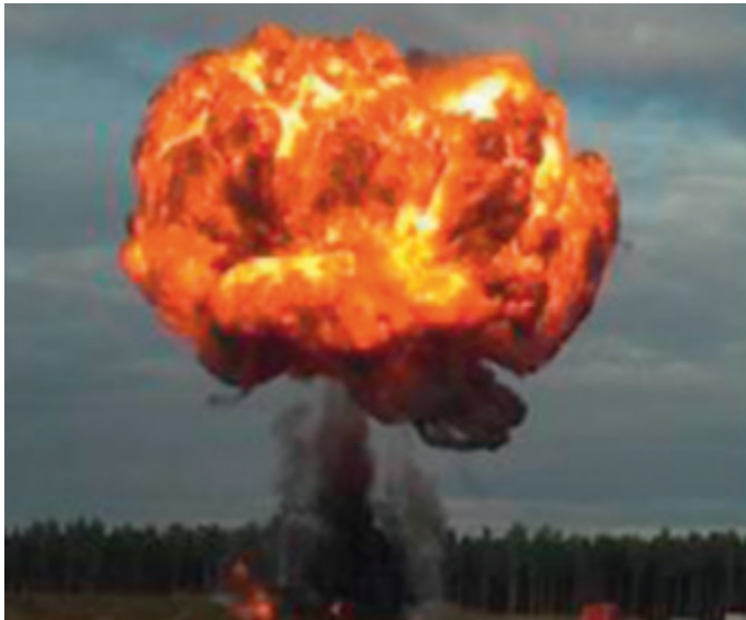
Example of a fireball created by a 900 L (238 gal) composite IBC (thermal decomposition phenomenon)
