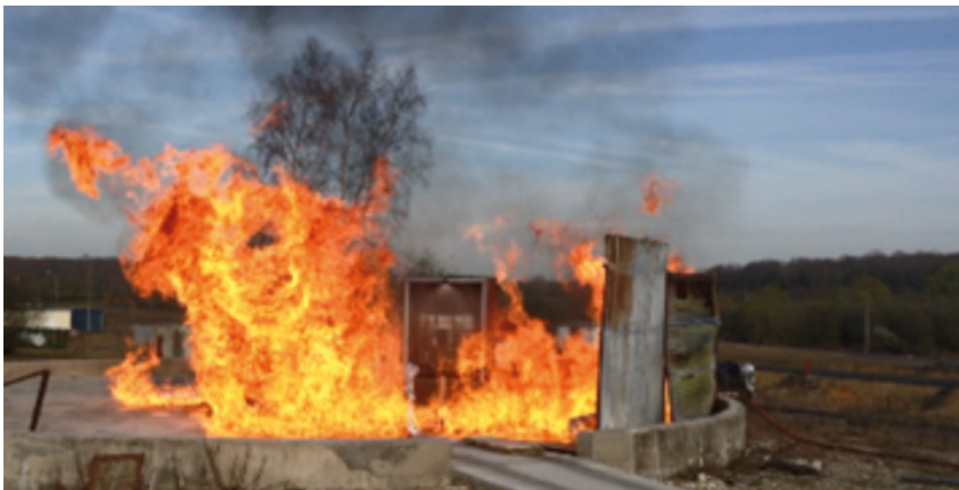
Pool fire during a test with an IBC filled with flammable liquid. Allianz ©
