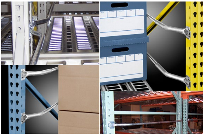
Physical Barriers Used to Maintain Flues
