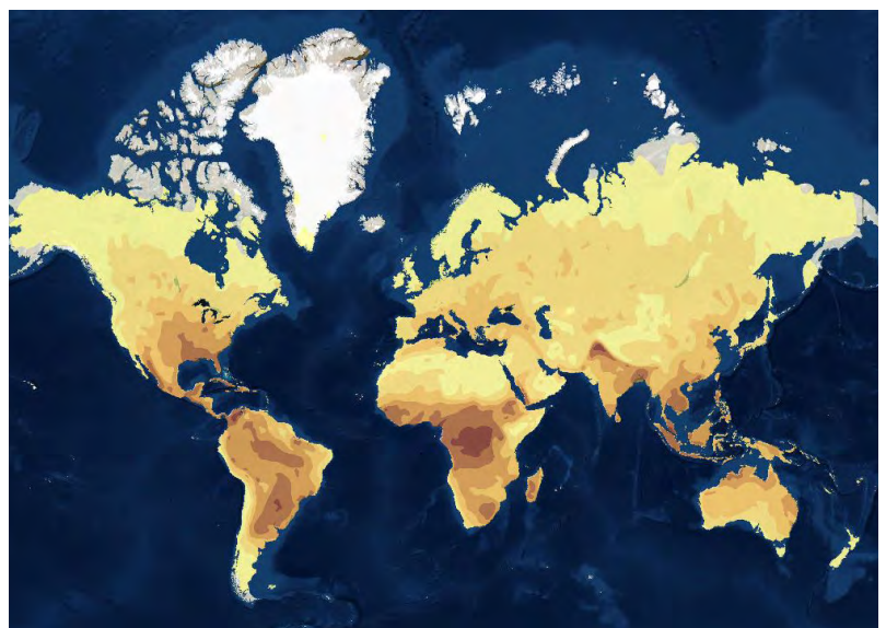
Munich RE map of global frequency of lightning strokes per km 2 and year
