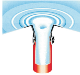
Air and water enter a gravity outlet
