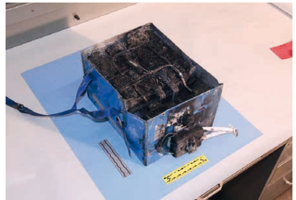
A heavily burned battery from an airplane after suffering thermal runaway. An increase in temperature changes conditions in a way that causes a further increase in temperature.
