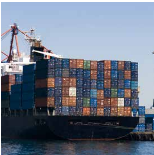
Safe working limits of machinery can be compromised by overloaded containers
