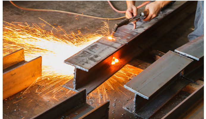
Hot work permits should be required for anyone performing hot work at the site
